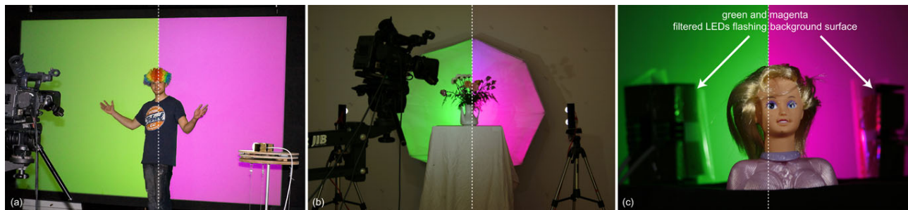
Fig. 5 Different prototype implementations of temporal backdrops: a backprojection screen (a), a softbox with integrated RGB LEDs (b), and a RGB front-illumination of a diffuse background surface (c). The foregrounds are lit with arbitrarily aligned spot lights
